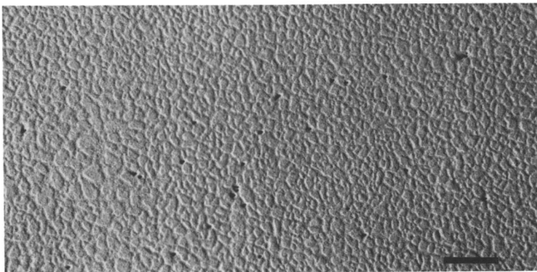
Figure 8. Polystyrene exposed to human serum albumin in the flow cell for 6 sec at 135/sec., then reacted with the anti-HSA antibodies conjugated with 20 nm. colloidal gold particles. The scale bar represents 100 nm.
