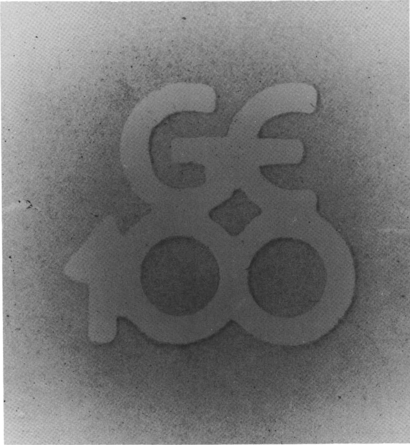
Figure 4b. Haptotactic behavior of WI-38 cells on a specially prepared glass coverslip. The background, showing normal cell-substrate interaction, is covered with a layer of adsorbed BSA, while the pattern (GE100) is covered with IgG molecules specifically attached to a base layer of BSA.
